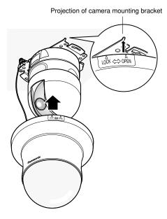
③ Turn this bracket clockwise until the projection of the camera mounting bracket aligns with "LOCK" of this bracket.
