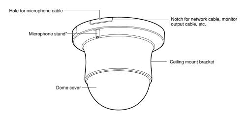
\* If a microphone is used, mount the microphone on the rubber-made microphone stand. Unless the microphone is used, cut the rubber with a nipper or conduct another treatment.
